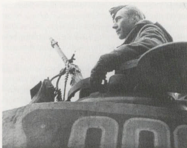
All crews were alert to the danger which constantly threatened them from a sky dominated by Allied tactical aircraft; an aircraft sentry was always on watch in every vehicle, and this photo shows the AA MG mount on Tiger '003'.
